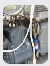
ECOGEL batch freezers are equipped with two parallel refrigeration systems that allow a reduction of 20% of nominal power applied and reduce, as a result, the consumption of energy and water. The emptied cylinder can be kept cold between + 1° C to + 3° C.
