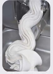
PRATICA models, like all VBF TELME batch freezers, have a vertical cylinder. Gelato is effectively mixed during preparation. The beater pushes the product upwards then gravity brings the product down again. The time controlled cycle allows for the rapid production of high quality gelato at the desired texture and consistency. The temperature cycle always allows to achieve the same result with different quanti-
